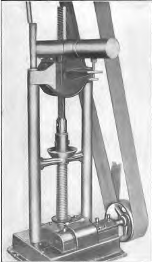
FIG. 62.—Vertical machine used for heavy rectangular broaching.]
